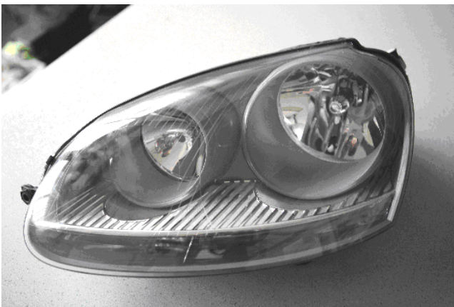
Fig. 3 Headlamp with H7 halogen filament lamp, with free form reflector and plain lens (VW Jetta).
