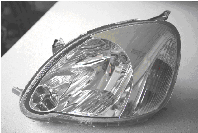
Fig. 2 Headlamp with H4 halogen filament lamp, with free form reflector and plain lens (Toyota Yaris)
