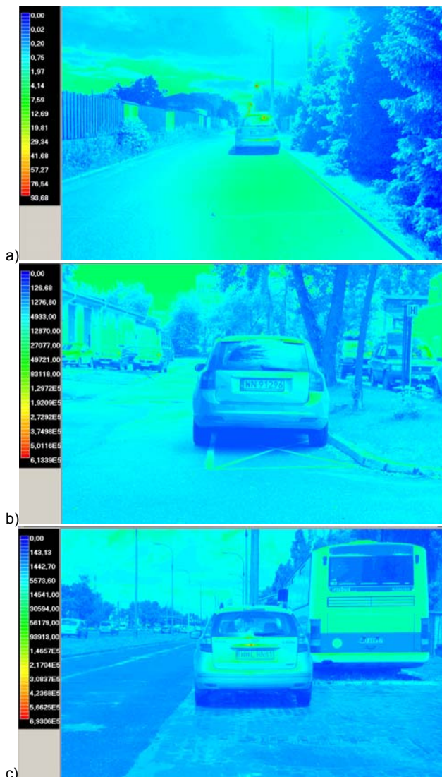
Fig. 4. Background luminance in typical road situations: a) 1,5 cd/m 2 ; b) 4600 cd/m 2 ; c) 7000 cd/m 2 + additional glare from the reflections of the car bodies
