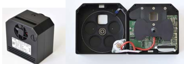
Fig. 3. Ventilator location for cooling Peltier cells and interior of CCD camera with disc for 5 filters
