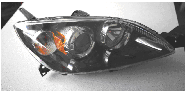
Fig. 3 Headlamp with H7 halogen filament lamp, with free form reflector and plain lens (VW Jetta).
