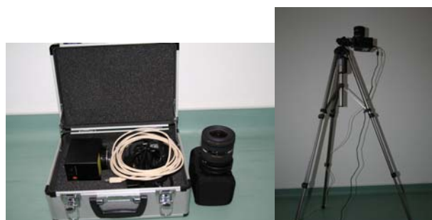
Fig. 1. CCD camera equipped with fisheye lens and placed on a tripod to capture the upper hemisphere luminance
