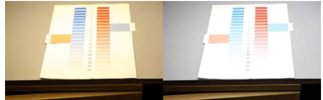
Figure 3b. The primary targets and the matching scales are shown at photopic lighting conditions ( L_p \approx 14 \text{ cd/m}^2 ). On the left hand side, the scenario under warm-white, on the right hand side under cool-white LED light is shown.
