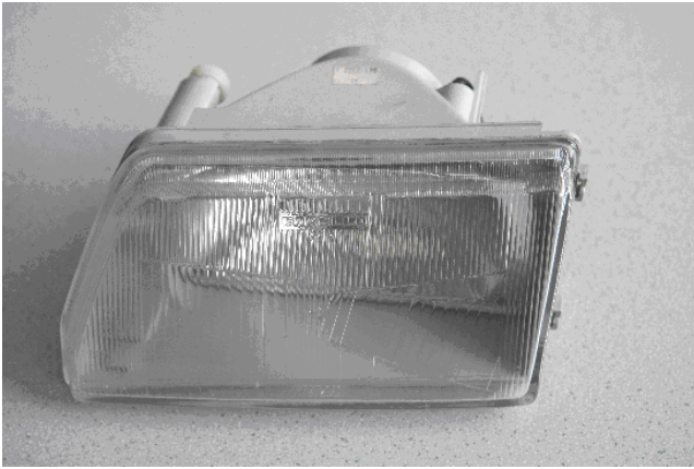
Fig. 1 Headlamp with H4 halogen filament lamp, with parabolic reflector and ribbed lens (Fiat Cinquecento)
